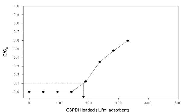
**Figure 4.** G3PDH adsorption performance in the UpFront contactor. The feedstock was previously disrupted by bead milling at 50 % w/v and was diluted to the equivalent of 25 % original wet cell weight pre-wet milling. The feedstock was applied to the expanded bed contactor at a constant linear velocity of 450 cm/h. Samples were centrifuged and assayed for enzyme activity which was expressed as  $C/C_0$ , where  $C_0$  = original activity and  $C$  = enzyme activity in samples.
