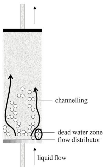
**Figure 1.** Diagram showing an uneven flow distribution of incoming feedstock. An uneven flow distribution of incoming feedstock will contribute to the formation of channelling and dead water zones in fluidised beds. Various types of devices including plates, mesh, glass beads and mechanical stirrer have been used as flow distributors.
