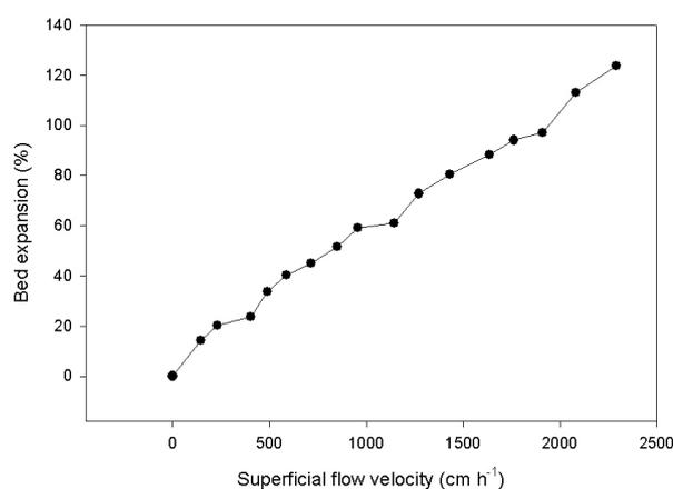
**Figure 3.** The bed expansion of UpFront Cibacron Blue 3GA as a function of superficial flow velocity of buffer A. Adsorbent particles (UpFront Cibacron Blue 3GA), corresponding to a settled bed height (SBH) of 15 cm were loaded into UpFront contactor. The degree of bed expansion was monitored visually as a function of increasing superficial velocity of buffer A.
